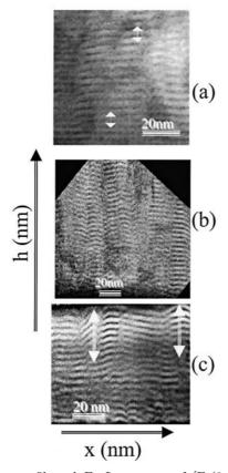
**Fig. 3.** Energy filtered Fe  $L_{2,3}$  maps of [Fe(3 nm)/Cr(1.2 nm)]<sub>n</sub>-superlattices. (a) Bilayers 3rd to 19th (4 mTorr); (b) bilayers 6th to 38th (5 mTorr); (c) bilayers 1st to 18th (10 mTorr). Arrows in (a) and (c) show the replication distance of small bumps and large bumps respectively. Scales in the growth direction are the same as that drawn over the micrograph in the lateral direction.
