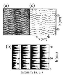
**Fig. 2.** (a) Typical Fe-map of [Fe(3 nm)/Cr(1.2 nm)]<sub>n</sub>-superlattice grown at an Ar-pressure of 5 mTorr. (b) Fe-profiles for 4 different integration windows, h is the coordinate in the growth direction. Symbols ( $\triangle, \square$ , O) identify the position of height maxima for each bilayer. (c) Bilayer profiles for superlattice shown in micrograph (a). Figures (a) and (c) are on the same scale.
