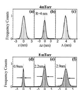
Fig. 4. Statistical plots of: (a) height function z(x), (b) height difference  $\Delta z(R) = z(x) - z(x+R)$  for R=4 nm, (c) bilayer modulation length  $\Lambda$  for an [Fe(3 nm)/Cr(1.2 nm)]<sub>20</sub> superlattice grown at 4 mTorr. Statistical plots of the height differences  $\Delta z(R)$  for: (d) R=1.35 nm, (e) R=4 nm, (f) R=6.7 nm for an [Fe(3 nm)/Cr(1.2 nm)]<sub>20</sub> superlattice grown at 8 mTorr. FWHM, indicated by arrows are 0.9, 2.2 and 2.9 nm respectively.
