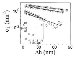
**Fig. 7.** The height-height correlation function in the growth direction  $c_{\perp}$ , as a function of vertical distance  $\Delta h$  for  $[\text{Fe}(3 \text{ nm})/\text{Cr}(1.2 \text{ nm})]_{20}$  superlattices grown at 4 (O),  $6\triangle$ ),  $8(\nabla)$  and  $10(\Box)$  mTorr. The inset shows the dependence of the roughness correlation length in the growth direction  $\xi_{\perp}$  as a function of pressure.
